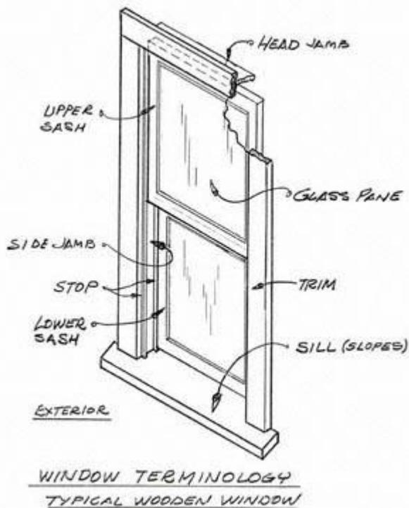
**Sash** – The framework holding the glass in the window.
